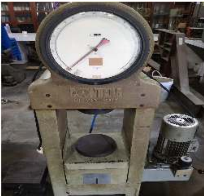
Gambar 3.3 Alat kuat tekan beton (CONTROLIS MILANO – ITAL
